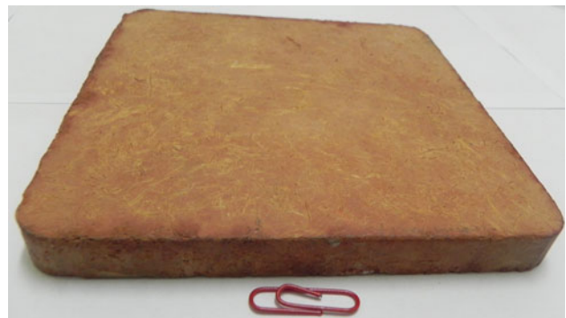
Fig. 2 Photograph of a 15-mm thick silica fibre-reinforced phenolic syntactic foam
